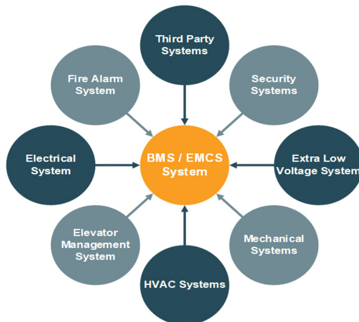
Figure 1: High-Level View of the Configuration of BMS and MEP Systems
